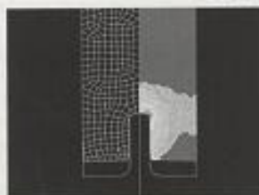
Fig. 14 — Simulation shows material moving into relief section of pin.
