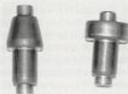
Fig. 12 — Forming sequence developed using NAGFORM and NAGSIM.2D.
