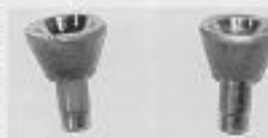
Fig. 6 — Formed part before (l), after (r) tooling changes.
