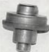
Fig. 9 — Formed part not filled at the corner.
