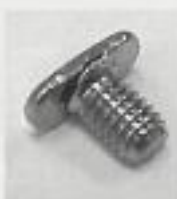
Fig. 3 — Cracked during assembly.
